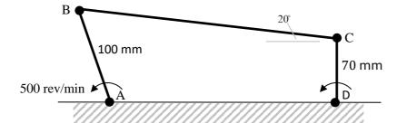
Calculate the angular velocity of the output crank.
