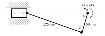
At the instant shown, calculate the magnitude and direction of the acceleration of piston C and the angular acceleration of connecting rod BC.
