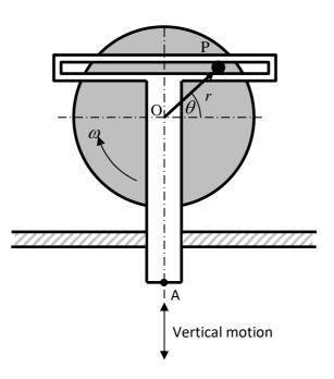
The pin is located at a radius r = 2 cm and the wheel has constant angular velocity  $\omega = 6 \text{ rad/s}$ , and at the instant shown  $\theta = 30^{\circ}$ .
