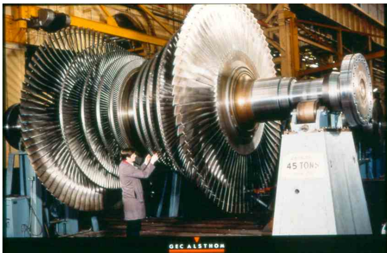
Fig 2. A typical low pressure steam turbine from Alstom as used in a power generation station.
