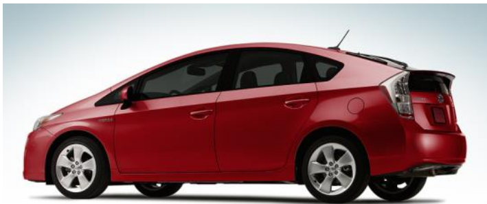
Figure 16: Car drag coefficients. a) Trend to 2000 [1]; b) Toyota Prius V [6], C_D = 0.25 ; c) Nuna [8], C_D = 0.07
