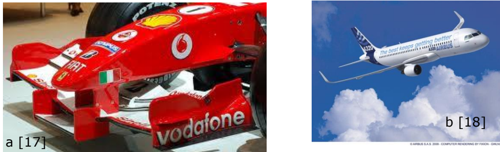
Figure 33: Endplates (a) and winglets (b) reduce induced drag.
