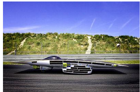
Figure 16: Car drag coefficients. a) Trend to 2000 [1]; b) Toyota Prius V [6], C_D = 0.25 ; c) Nuna [8], C_D = 0.07
