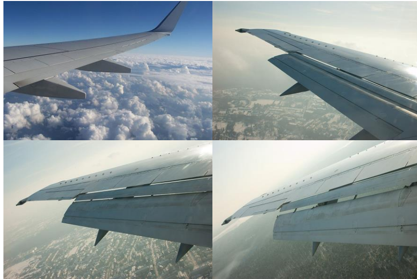
Figure 26: wing flaps on a Boeing 737 shown going from retracted to fully extended for landing [19]
