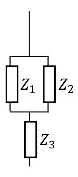
Break the circuit up into series and parallel and solve individually
