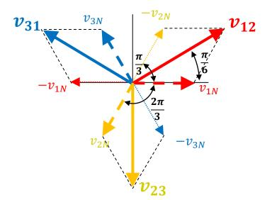
$|v_{12}| = |v_{23}| = |v_{31}| = \sqrt{3}|v_{1N}| = \sqrt{3}|v_{2N}| = \sqrt{3}|v_{3N}|$ |Line Voltage| =  $\sqrt{3} \times |Phase Voltage|$  $415V = \sqrt{3} \times 240V$
