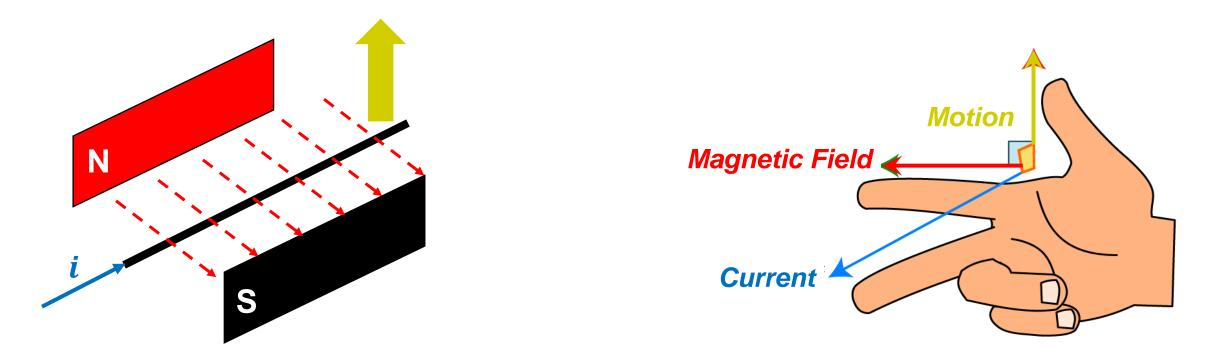
A conductor moving in a magnetic field generates a voltage across itself (current produced if circuit was to be completed)
