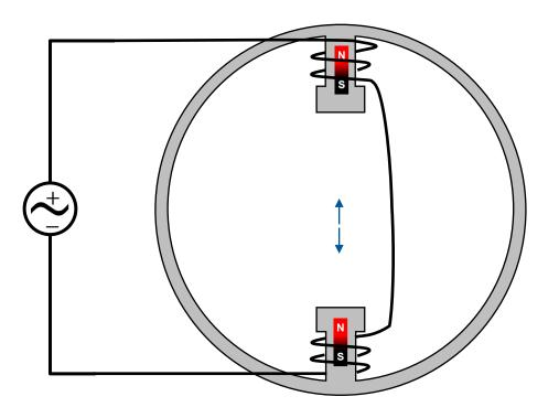
But, with a single pair of poles and single phase AC, we only get a single dimension of motion
