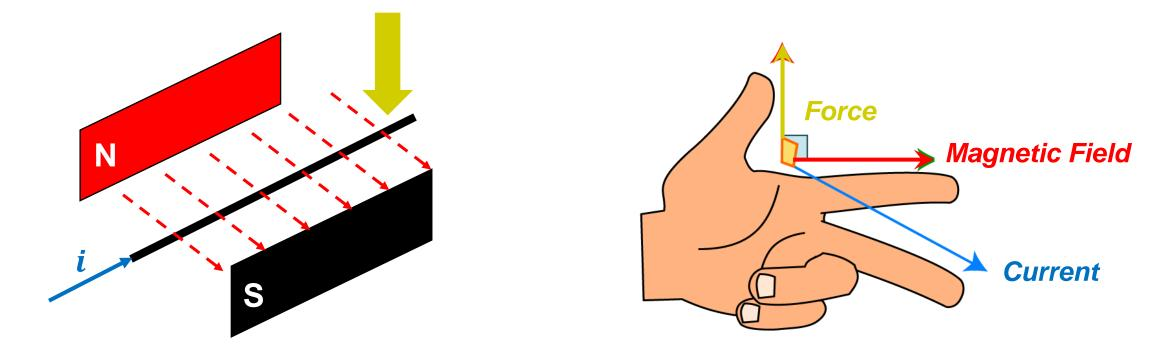
A current-carrying conductor in a magnetic field experiences a force/thrust
