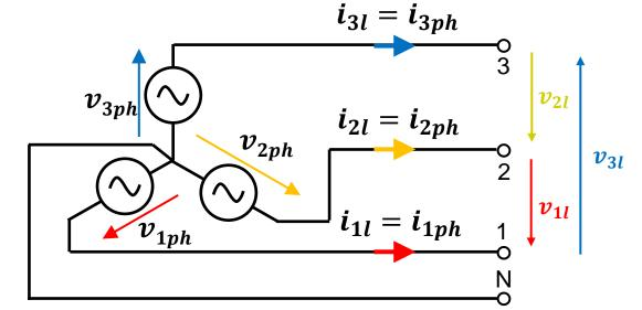
Relationship between phase and line voltages for star-connected device?
