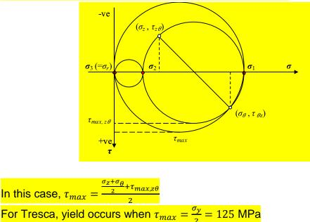
University of Nottingham Department of Mechanical Engineering Therefore, when  $120 + \tau_{max,z\theta} = 250$  MPa or  $\tau_{max,z\theta} = 130$  MPa which is not a feasible solution as the minimum principal stress in this plane would then be *C* - *R* = 120 - 130 = -10 MPa, which is less than  $\sigma_r = 0$
