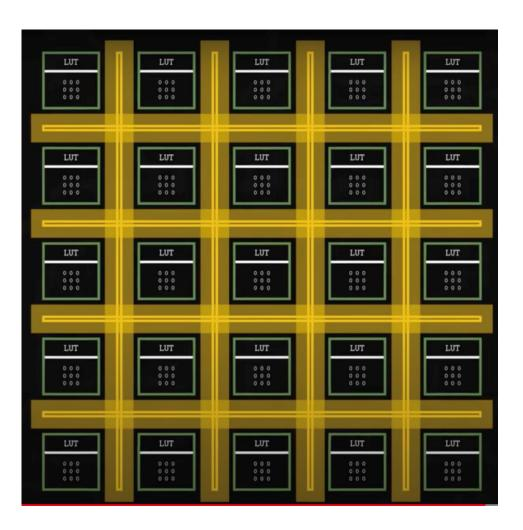
This can be done through routing fabric between the LUTs
