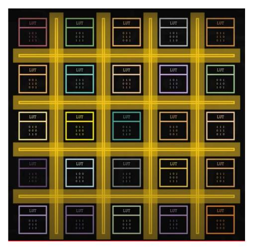
Now by programming the LUTs and re-wiring them, we can do any combinations of arithmetic or complex process!!
